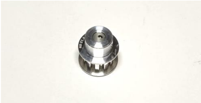
Qty.(1) XL 10 tooth 6mm bore pulley
