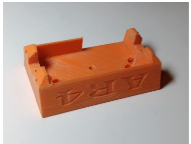
AR4_SG1_carriage (3D print – PETG 50% infill)
