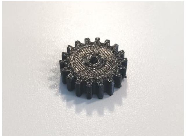
AR4_SG1_gear (3D print – PETG 50% infill)
