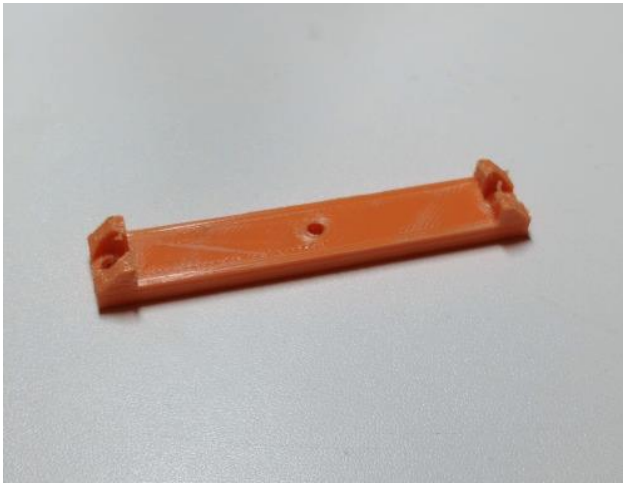
AR4_SG1_center_bar (3D print – PETG 50% infill)
