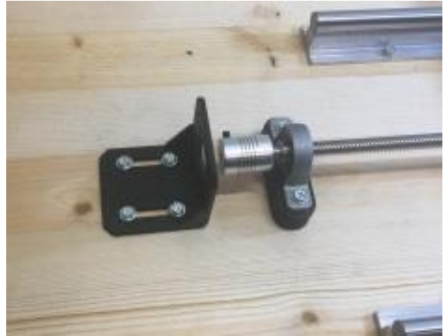
Remove motor and secure motor mount to work table as shown.
