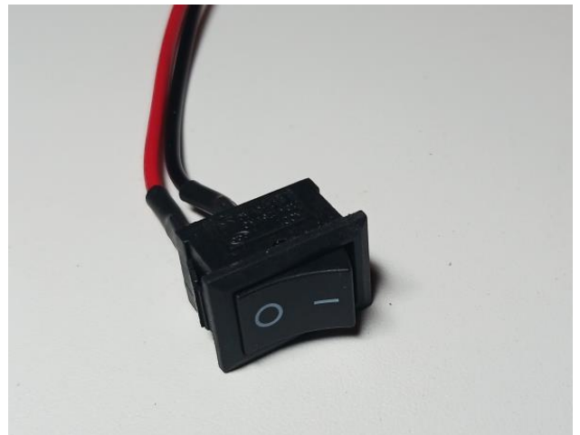
KCD1 SPST rocker switch with lead wires.
