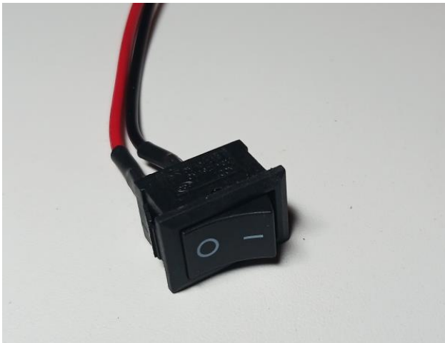
KCD1 SPST rocker switch with lead wires.
