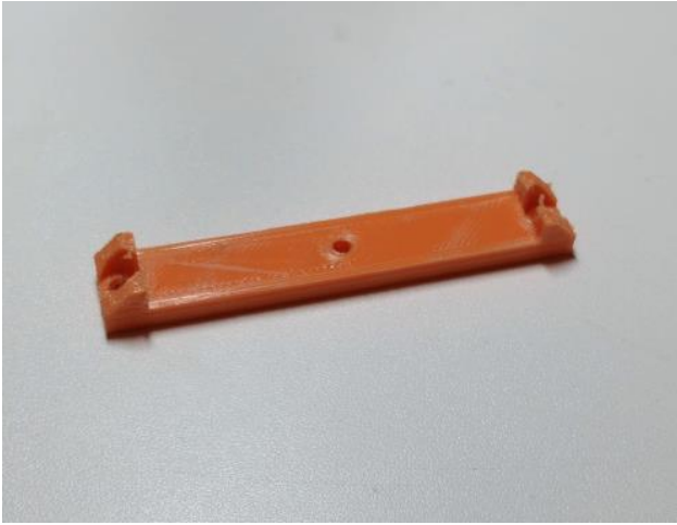
AR4_SG1_center_bar (3D print – PETG 50% infill)
