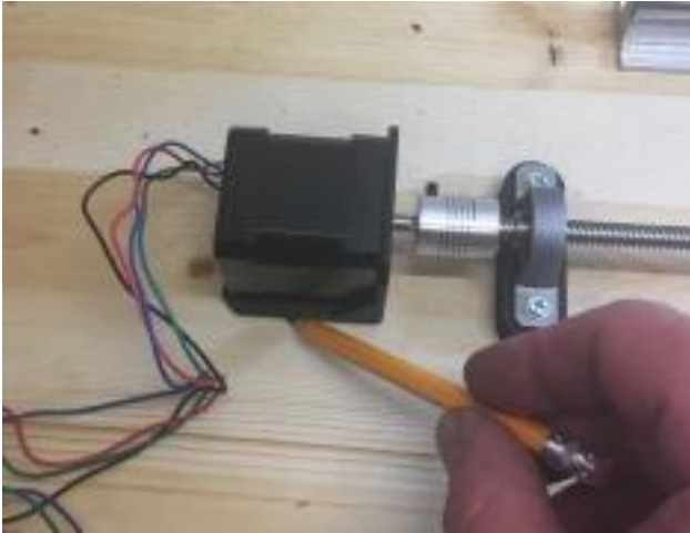
Temporarily install motor and bracket and use pencil to mark motor mount location.
