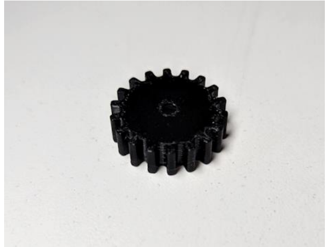
AR4_SG1_gear (3D print – PETG 50% infill)
