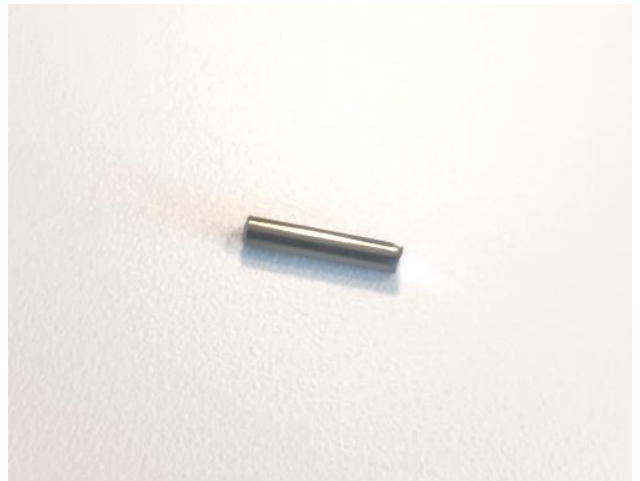
3mm stainless rod cut to length of 16.5mm
