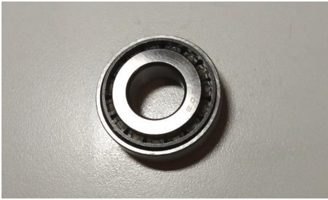
Qty.(1) 30203 (17x40x13.25mm) taper roller bearing.
