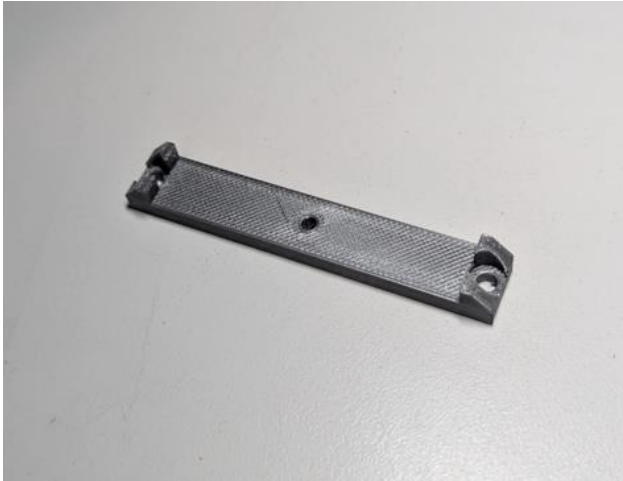
AR4_SG1_center_bar (3D print – PETG 50% infill)
