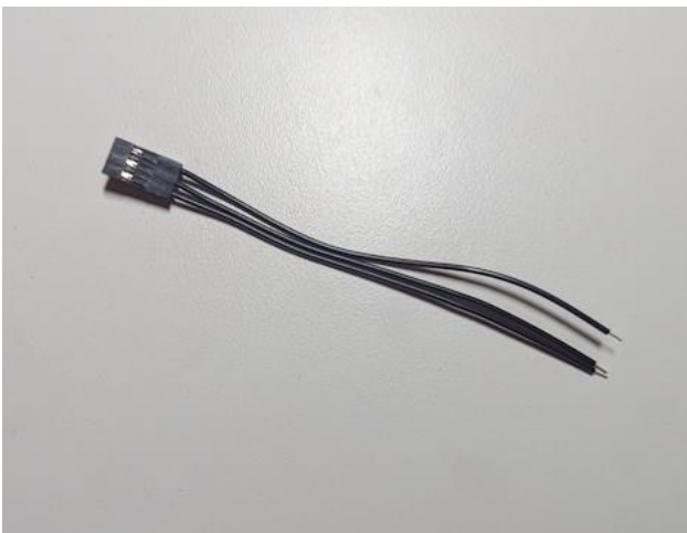
Dupont 2.54 mm female 3 pin connector lead.
