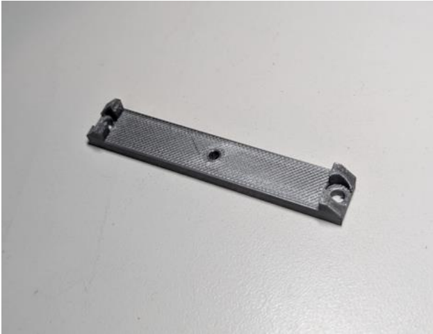
AR4_SG1_center_bar (3D print – PETG 50% infill)
