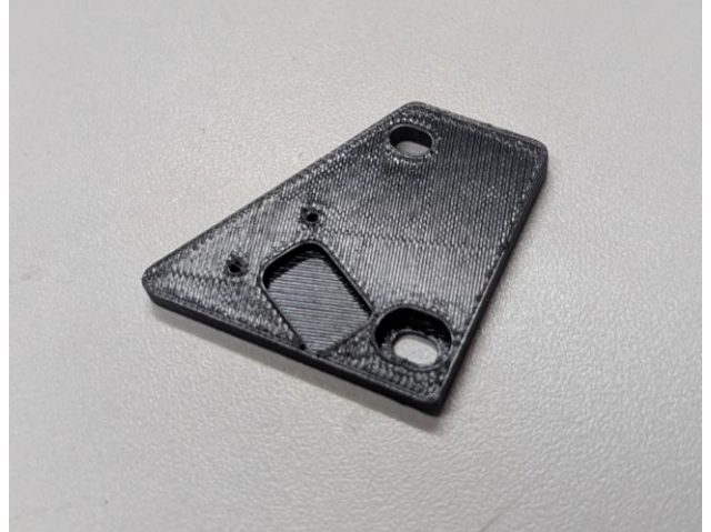
MK4 TO MK5 J2 SENSOR MOUNT PETG FILAMENT 15% INFILL 2X WALLS
