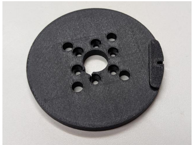
MK4 TO MK5 J2 TENSION RING ABS-GF FILAMENT 100% INFILL 4X WALLS
