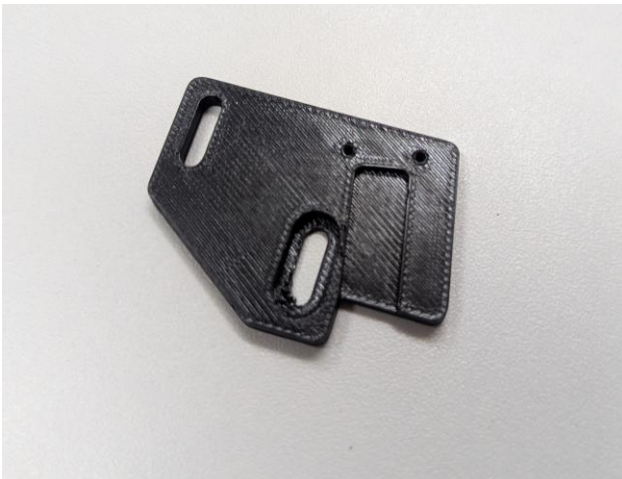
MK4 TO MK5 J3 SENSOR MOUNT PETG FILAMENT 15% INFILL 2X WALLS
