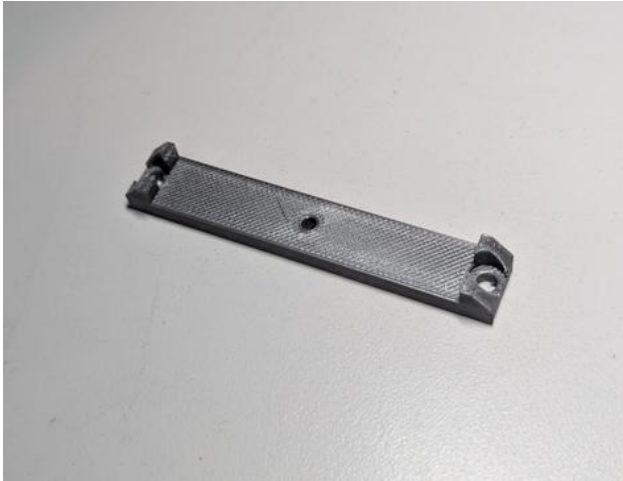
AR4_SG1_center_bar (3D print – PETG 50% infill)
