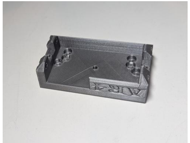
AR4_SG1_carriage (3D print – PETG 50% infill)
